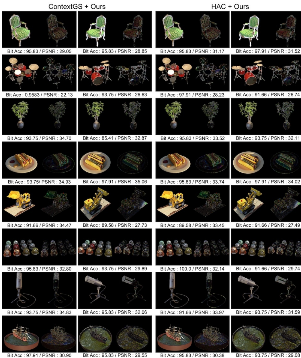
Figure 16: Rendering quality of various rendering outputs generated by our method on the Blender dataset. We show the differences ( \times 5 ). The closer it is to white, the greater the discrepancy between the ground truth and the rendered image. The results were obtained using 48-bit messages after compression.
