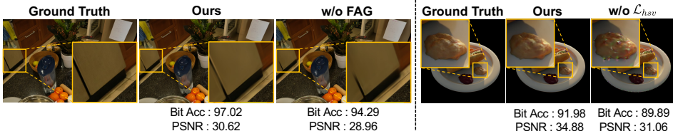
Figure 6: Qualitative comparison of rendering quality with full method (ours), without FAG (left), without \mathcal{L}_{hsv} (right). Rendered images are obtained with 48-bit watermark embedding.
